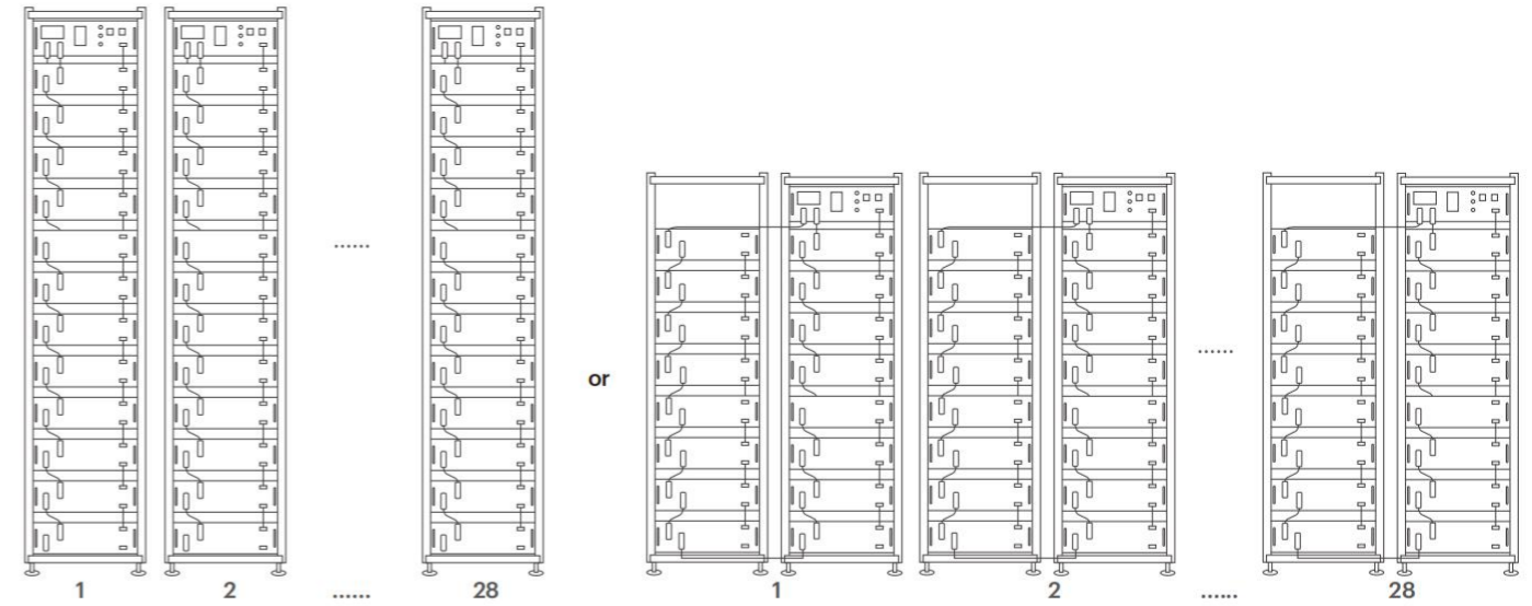
Maximum support for 28 clusters of batteries in parallel
